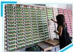
9. Aging test for travel charger
